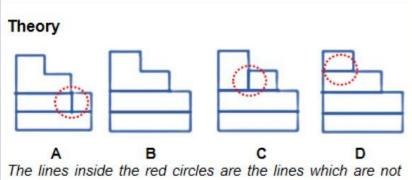
The lines inside the red circles are the lines which are not possible in the front view. So Option B is correct
